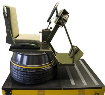
The vehicle model takes into account spring and damping rates, bump stops, anti-sway bars, anti-squat anti-dive geometry, and roll axis height.
