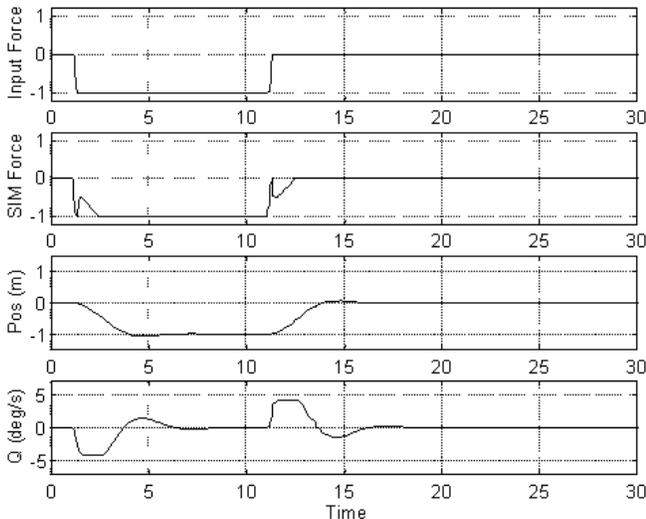
This example is the same size motion base with the same tuning parameters as above responding to a 0.5 m/s/s acceleration. (The non-linearity of the algorithm in this case eliminating the sagging and false cues).
