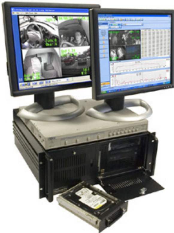
SimObserver hardware showing quad view, Data Distillery interface and removable hard drive.
