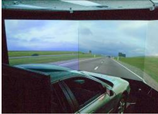
Half cab driving sim with three channel display.
